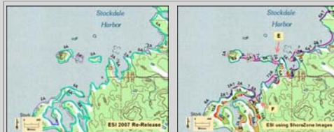
Figure 7. Stockdale Harbor, Montague Island. Left: Shoreline types from ESI 2007 re-release digital files. Right: Shoreline types determined using ShoreZone images. "E" and "F" refer to ShoreZone images in Figure 8.
